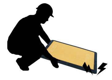
When fitting the product in place, never drop the product, gently lower it in place. Never lift or move with machinery. Never walk the product leading edge.
