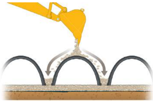
Figure 20 - Backfill Placement with Excavator
