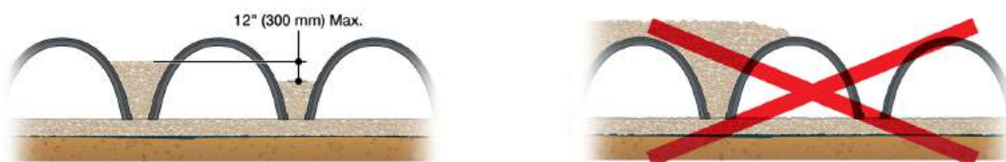
Figure 21 - Embedment Stone Placement
