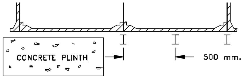
Standard base tanks (internally flanged base panels) may be laid directly on a concrete plinth having a trowelled finish, brushed clean and free from any local protuberances. It should be flat, level and not vary more than 6 mm in any 6 m, measured laterally or diagonally with a maximum variance of 2 mm per metre. The plinth must exceed the nominal tank dimensions by a minimum of 175 mm.
