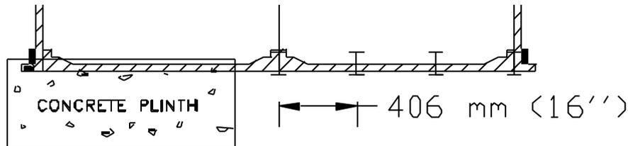
Standard base tanks (internally flanged base panels) may be laid directly on a concrete plinth having a trowelled finish, brushed clean and free from any local protuberances. It should be flat, level and not vary more than 6 mm in any 6 m, measured laterally or diagonally with a maximum variance of 2 mm per metre. The plinth must exceed the nominal tank dimensions by a minimum of 175 mm.
