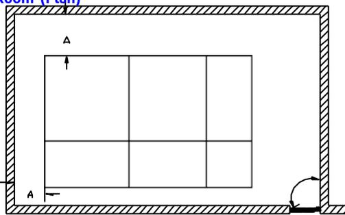
For dimension 'A' see chart below. This clearance should be on all sides of the tank, also a top clearance of 650 mm is required for standard access hatch to open. (This can be reduced to 450 mm provided that Killarney Plastics Ltd is notified prior to dispatch). If the tank has to be pushed closer to any wall after assembly or if the working space is reduced (dimension 'A') at a later stage, by the building of walls etc, responsibility will rest with others.
